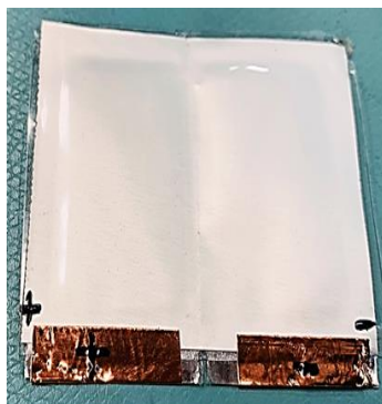
Figure 1: Schematic structure and fabricated supercapacitor
